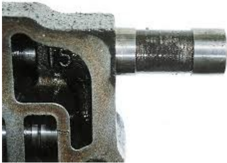
Valve body spool with heavy deposit build-up.
