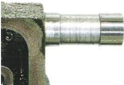
Valve body spool after transmission service.
