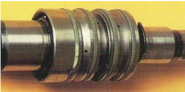
Power steering spool valve and hardened, cracked seals.
