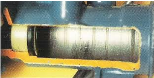
Grooves are worn into the soft metal of the spool valve housing by hardened seals. Metallic debris from such wear accumulates in the fluid causing premature component failure!
