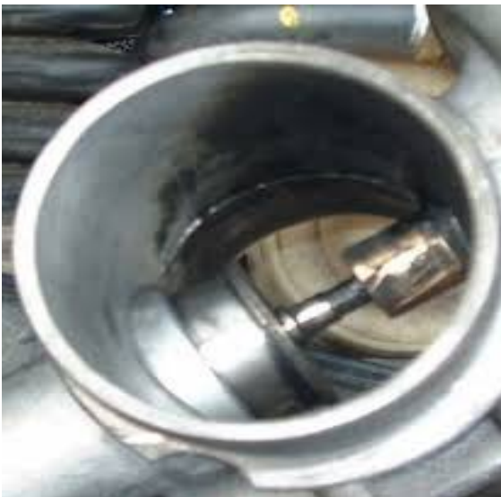
EGR ports are clean, harmful exhaust emission reduced, engine performance is improved.
