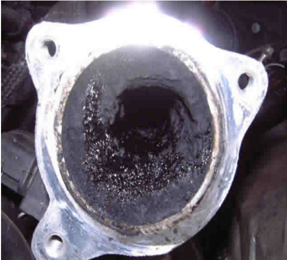
EGR ports become clogged with heavy carbon, exhaust emissions increase, engine performance is reduced.
