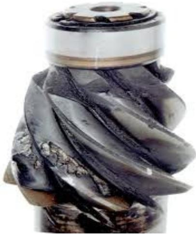
Lubricant breakdown can severely damage critical gear components!
