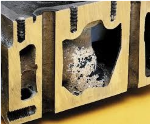
Severe corrosion which can occur when additives that protect the Cooling system have been depleted.
