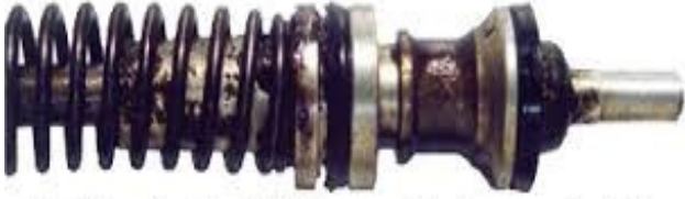
Harmful deposits and varnish build-up ---- resulting from worn-out, oxidized brake fluid ---- are apparent on this brake master cylinder piston assembly.
